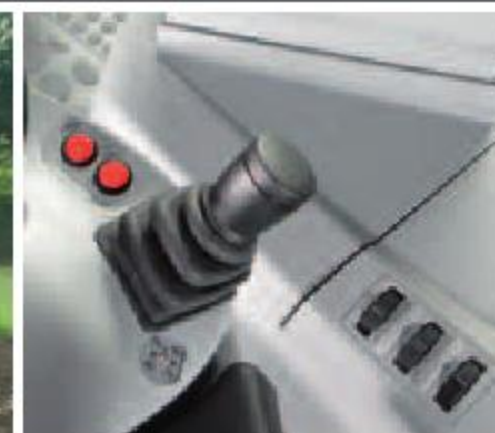
Maximum practical convenience in controlling the main functions of the auxiliary spool valves.
