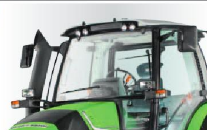
Twin pairs of lights incorporated at roof level, with extra wide beam provided by 14 powerful halogen lamps (Xenon lamps also available as optional accessory) able to illuminate a cultivation area of 600 m 2 .
