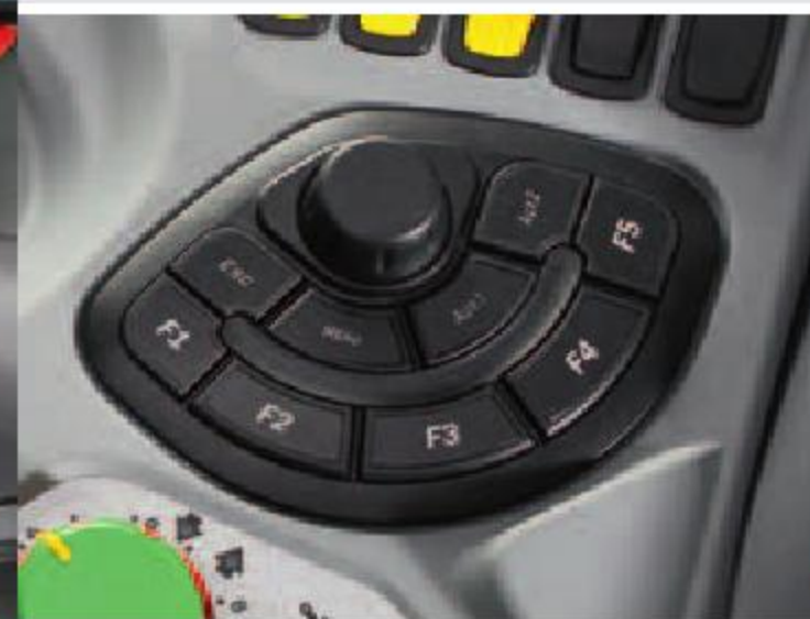
With the control panel located on a console to the right of the driving position, the operator can navigate easily through the menus using the dial.
