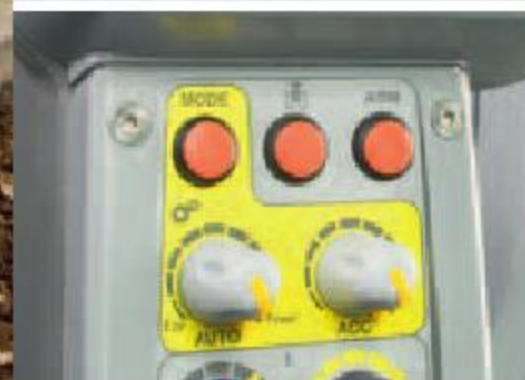
A button and two dials on the multifunction armrest are used to activate and control the various driving strategies, combining transmission and engine settings to best advantage.
