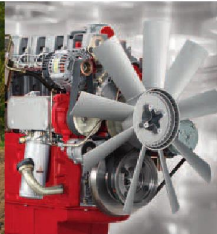
The electronic control viscous fan (E-Visco-fan) operates at variable speeds depending on the temperatures and the loads. It is a low energy consumption system which is activated only when needed.
