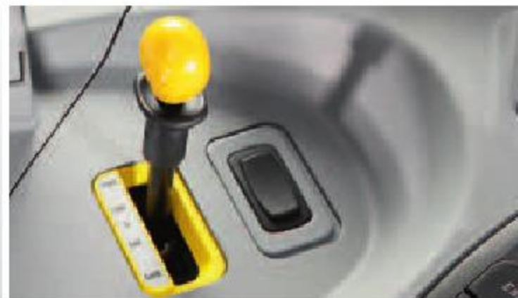
The PTO speed is easily changed by operating the yellow lever to the right of the driving position.
