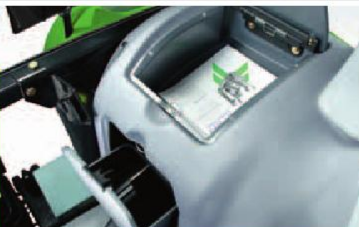
The drinks cooler compartment runs off the air-conditioning system and can hold 1 large bottle (2 litres) + 1 can. The storage compartment has a capacity of 7 dm 3 and will accommodate a DIN standard first aid box.
