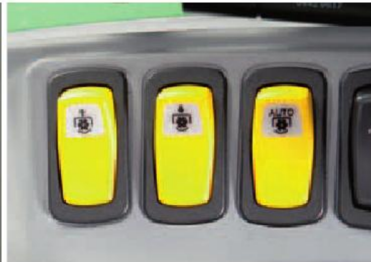
In PTO auto mode, the rear power take-off is deactivated the moment the rear lift comes into operation.
