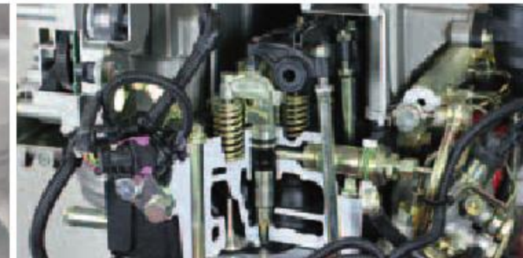
The 16 valve distribution permits a perfect filling of the cylinder and an optimization of the air-diesel oil mixture.
