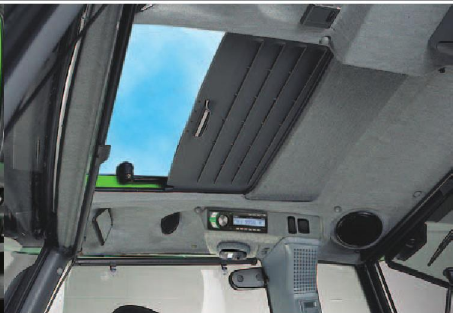
A generously proportioned glass roof hatch, with sunshade, allows excellent visibility when using a front loader.
