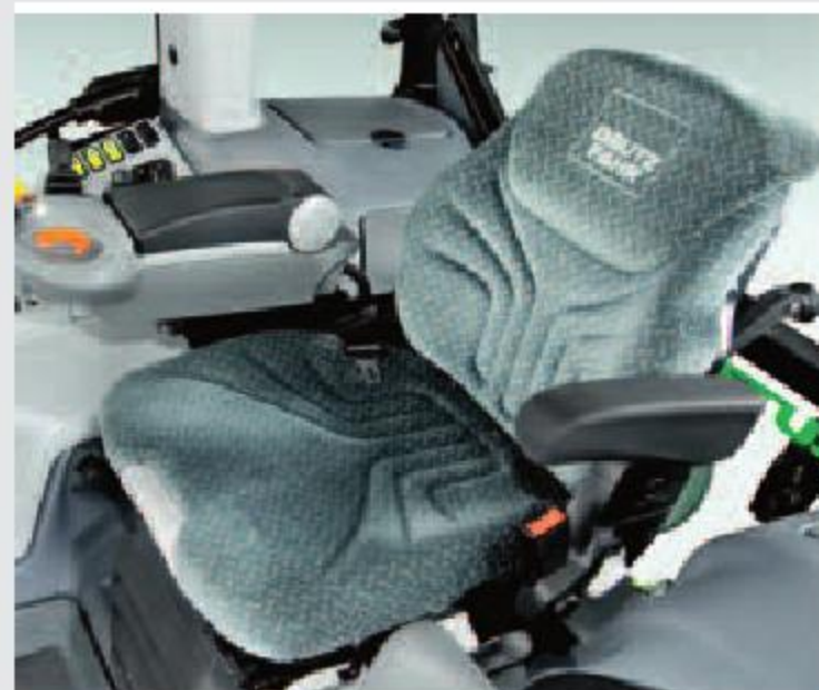
The driver's seat with Deluxe pneumatic suspension is generously sized, the wrap around type, covered in nonslip fabric.
