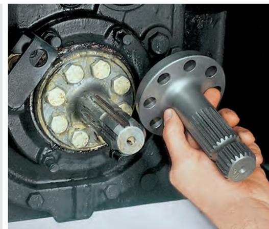
Fast replacement: The screw-connection PTO stub.
