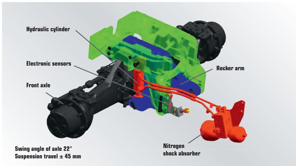
Comfortable and safe: The Agrotion M has hydro-pneumatic front axle suspension.
