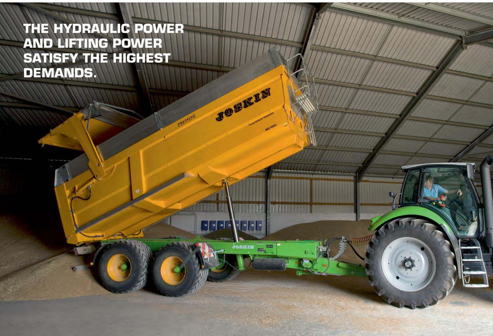
**You can never have enough hydraulic power. With this in mind the Agrotron M is fitted as standard with closed center loading sensing hydraulic system which satisfies the very highest demands with a delivery rate of 120 l/min and a system pressure of 200 bar.**
