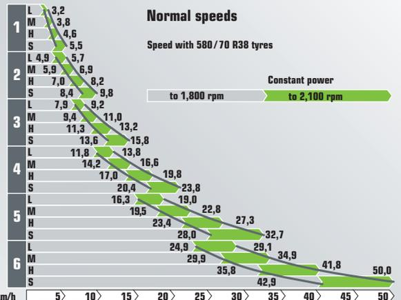
Economical in each speed: Additional Powershift stages are unnecessary due to the perfect coordination of engine and transmission. The driver can drive without constant shifting and still save fuel.
