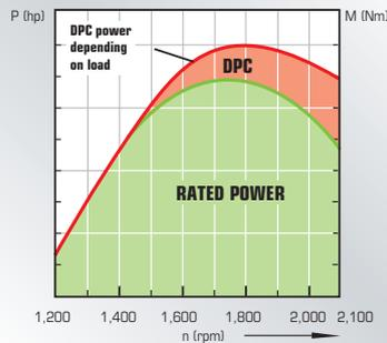
**DEUTZ-FAHR Power Control (DPC).** The innovative DPC technology delivers the highest and most economically efficient power at all times depending on the load situation. Strong torque, quick response characteristics and sufficient traction are therefore guaranteed even under the most difficult operating conditions.
